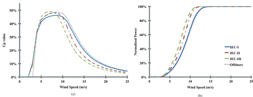
**Figure 1.** (a) The coefficient of power and (b) the normalized power curves for four generic IEC wind classes.
